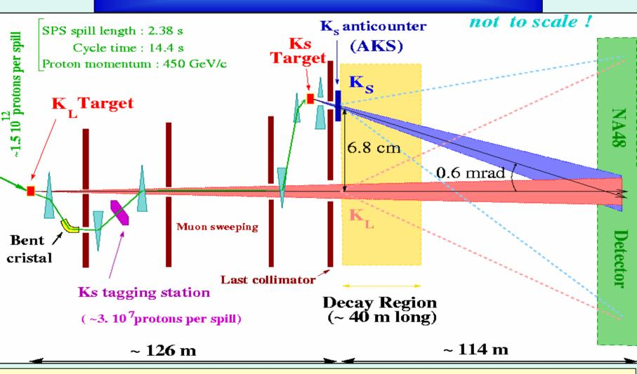
$K_s$  and  $K_L$  beams are distinguished by proton tagging upstream of the  $K_s$  target
