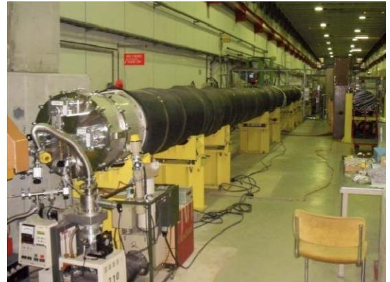
Fig. 6. The RICH prototype tested at CERN in 2007 and 2009
