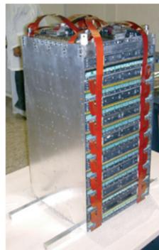
*One of the Large Area Telescope towers, which is composed of a stack of interleaved planes of silicon strips and tungsten converters. The LAT has 16 of these towers in a 4x4 array.
