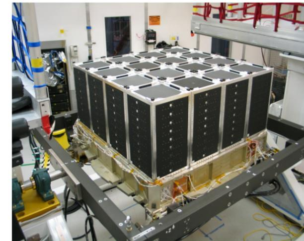
*The LAT has 16 towers of particle detectors, seen here before the installation of the Anticoincidence Detector. Each tower contains a Tracker module and a Calorimeter module. The Data Acquisition System is located underneath the towers. Credit: SLAC*
