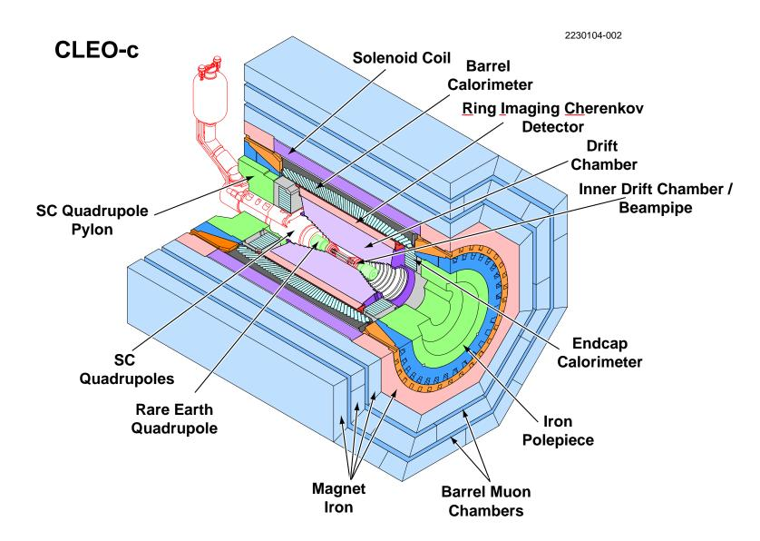
RICH for particle ID. Charged particle resolution  $\Delta p/p \simeq 0.6\%$  at 1 GeV/c; CsI calorimeter resolution 2.2% for  $E_{\gamma}=1$  GeV and 5% at 100 MeV. Inner drift chamber: all stereo.
