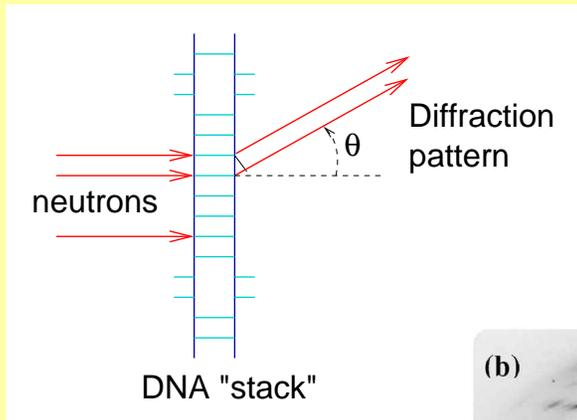
Measure the coherence length of the base stacking, which makes a diffraction grating.
