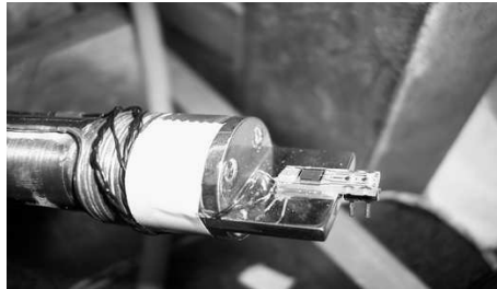
Fig. 1. – Cold finger liquid nitrogen cryostat and SiPM-thermometer glued
