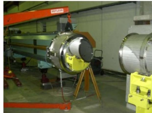
2009 test beam: RICH prototype with 414 PM
