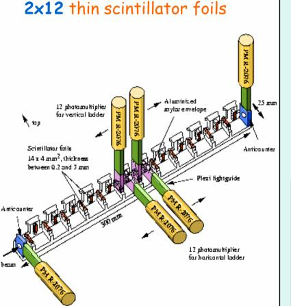
⇒ Proton rate ≈ 30MHz → split the intensity between foils, readout by 8 bits Flash ADC at 960 MHz
