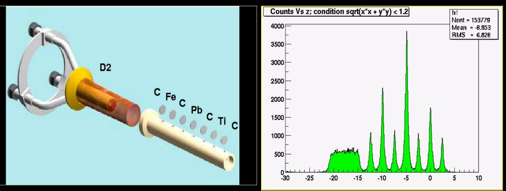
Proper spacing 2.5 cm to reduce multiple scattering
