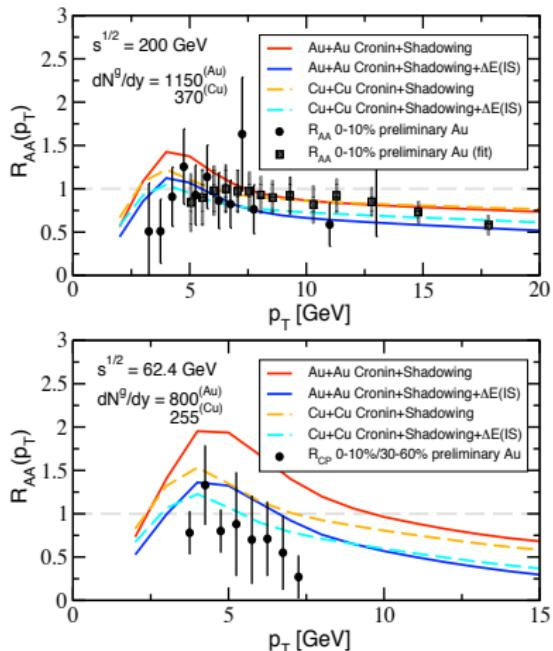
The contribution of the final-state photon production at  $p_T < 5 \text{ GeV}$  is limited to 35%, and at high transverse momenta, the modification of the direct photon cross section is dominated by initial-state cold nuclear matter effects.
