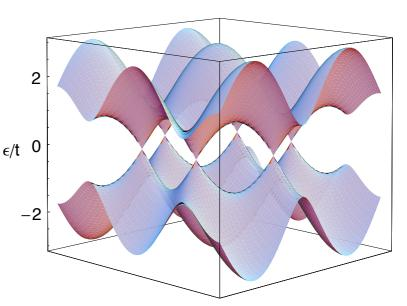
Half-filling (neutral or "undoped" graphene) has zero energy at "Dirac points" at corners of first Brillouin Zone:
