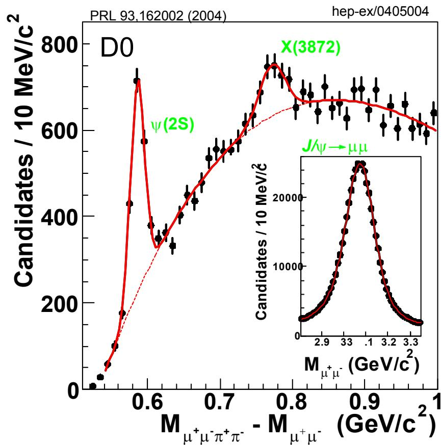
$$\begin{aligned}\Delta M &= 774.9 \pm 3.1(\text{stat}) \pm 3.0(\text{syst.}) \text{ MeV}/c^2 \\ \sigma &= 17 \pm 3 \text{ MeV}/c^2\end{aligned}$$
