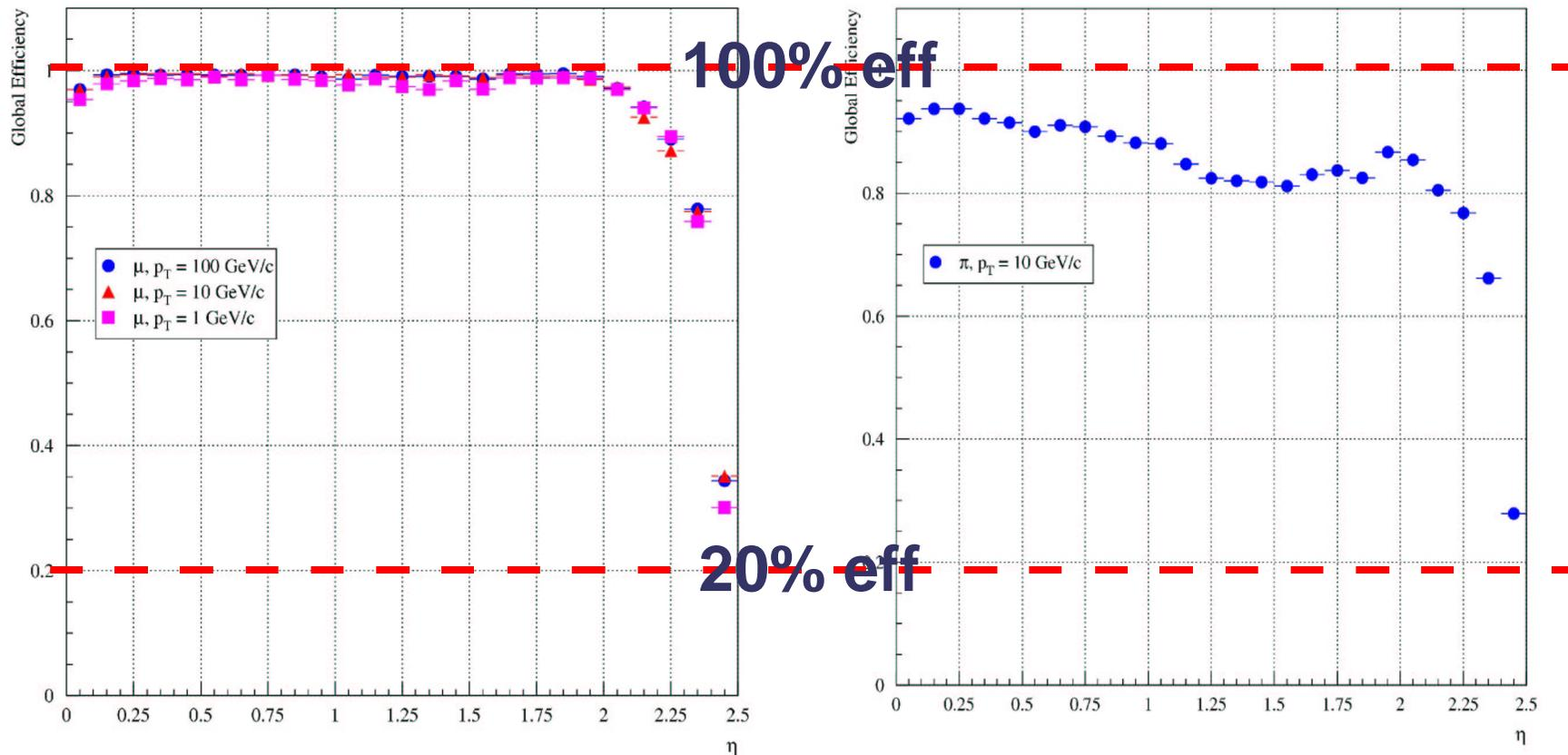
Lower reconstruction efficiency for Pions due to nuclear interactions inside the tracker (~20% of 1 GeV pions do not reach the outer layer).
