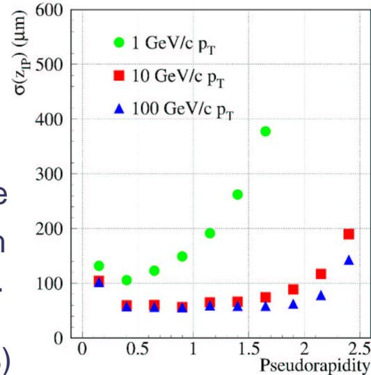
$\sim 60$   $\mu\text{m}$  of longitudinal impact parameter resolution for  $p_T = 1-10$  GeV/c in the barrel. (Full track reconstruction  $\sim 40\mu\text{m}$ )
