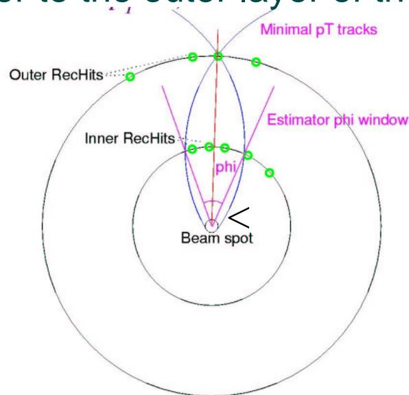
Initial trajectories (*seeds*) made of **pixel hit pairs**: every combination of 2 pixel layers, compatible with the beam spot and a minimum  $p_T$  cut.
