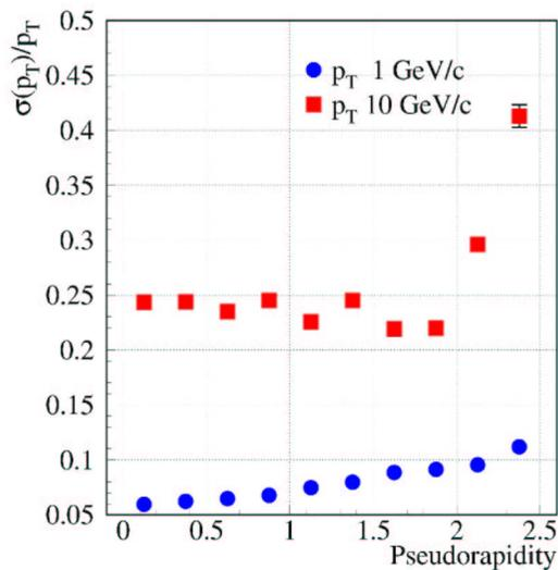
Degradation of high  $p_T$  measurement due to the short level arm of the Pixel Detector. (Full track reconstruction  $\sim 2-3\%$ )
