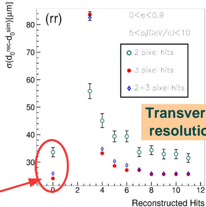
Good track parameter resolutions are obtained using only 5-6 hits compared with the full track reconstruction.
