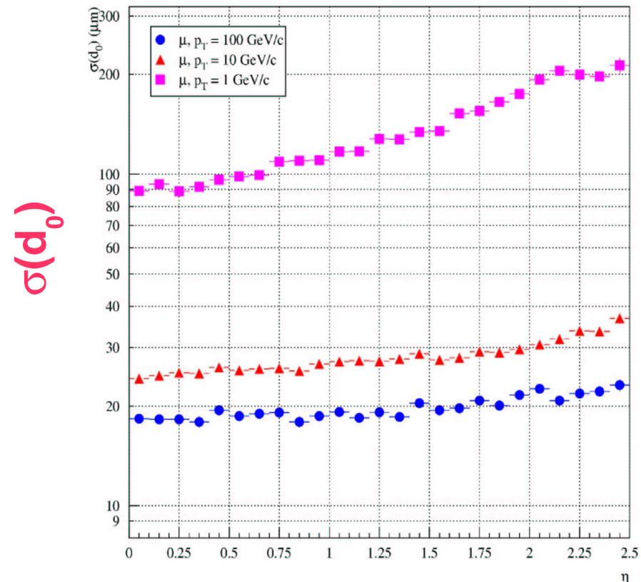
Resolutions mainly dominated by the level arm ( $p_T$ ) and the spatial resolution in pixel measurements ( $d_0$ ).
